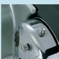
The Free-Fall technology applied to the Genius windlass allows free running of chain through the gypsy when lowering the anchor; simply by depressing the down control button the windlass will release its clutch and the gypsy will freewheel. To stop the Free-Fall depress the up control button on the windlass; the clutch will engage stopping the gypsy and allowing retrieval of the chain. The Free-Fall function can be bypassed to facilitate power controlled release.
